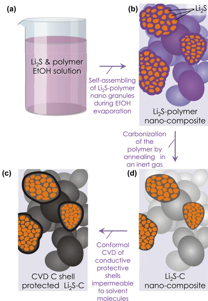
**Figure 3.** Schematic of the process flow for the scalable formation of hierarchical C-Li<sub>2</sub>S-C nanocomposite nanoparticles, involving both wet chemistry and vapor deposition approaches.
