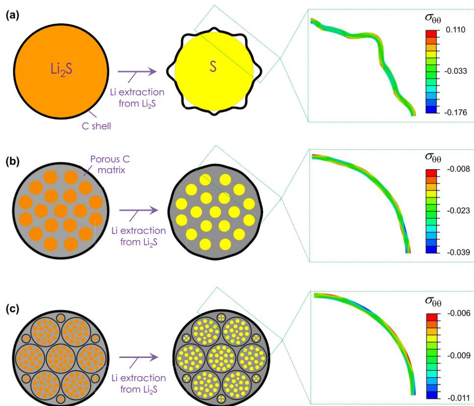
**Figure 2.** Results of the numerical modeling, showing significant reduction of the hoop stress (normalized by Young's modulus of carbon) within the outer shells of the  $\text{Li}_2\text{S}$ -C composite particles with the increasing level of the hierarchy in particles' shelling: a) zero level; b) first level; c) second level.
