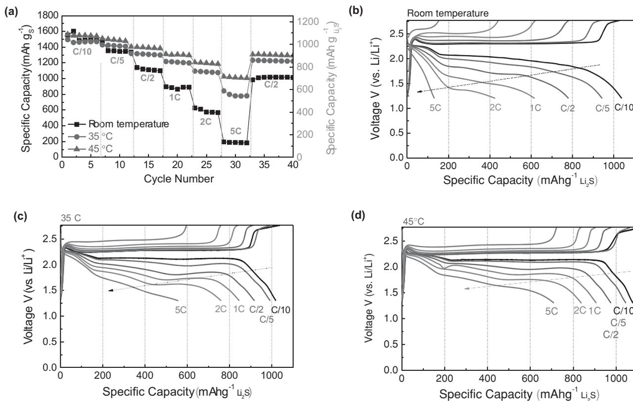
**Figure 6.** Electrochemical characterizations of the hierarchical C–Li<sub>2</sub>S composite nanopowder samples: a) discharge capacity at different C-rates and temperatures; b,c,d) charge–discharge profiles corresponding to different C-rates and recorded at: b) room temperature, c) 35 °C, and d) 45 °C.
