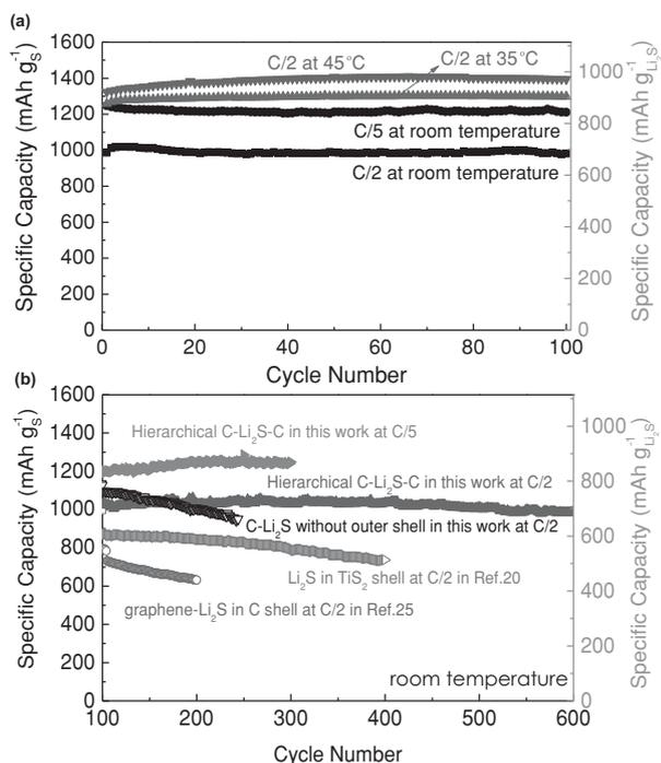
**Figure 7.** Electrochemical characterizations of the hierarchical C–Li<sub>2</sub>S–C nanocomposite nanopowder samples: a) cycling performance at C/2 and C/5 rates at selected temperatures, b) capacity and cycle stability of the produced samples with and without shells in comparison with previous literature reports on shell-enclosed Li<sub>2</sub>S powders.
