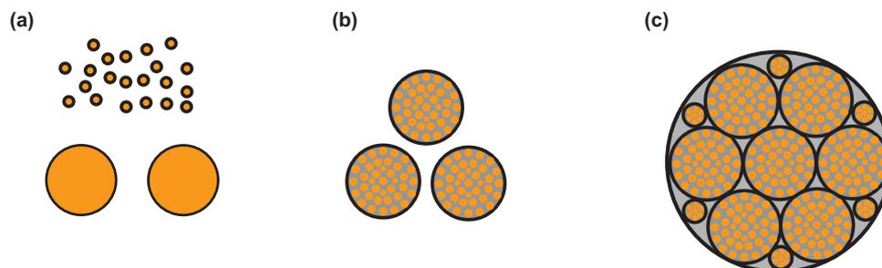
**Figure 1.** A concept of hierarchical particles' shelling for enhanced mechanical stability of volume-changing active materials, such as  $\text{Li}_2\text{S}$ . Particles exhibiting three levels of enclosing hierarchy are shown: a) zero (small and medium size particles), b) one, and c) two. Failure of a shell in a primary particle in (b) could be mitigated by a second-level shell. Failure of both a primary shell and a second-level shell in (c) could be mitigated by a shell at the third level.
