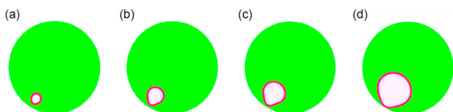
Figure 3. Phase field modeling of void nucleation and growth during the delithiation of GaND. The green region represents the matrix phase, the white region the void phase, and the red curve the interface. The void nucleation and morphologies resemble those seen in Figure 2.
